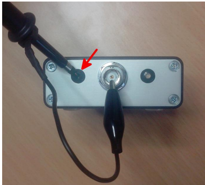
Monitoring Nominal Frequency; the red arrow indicates the frequency monitor terminal.
