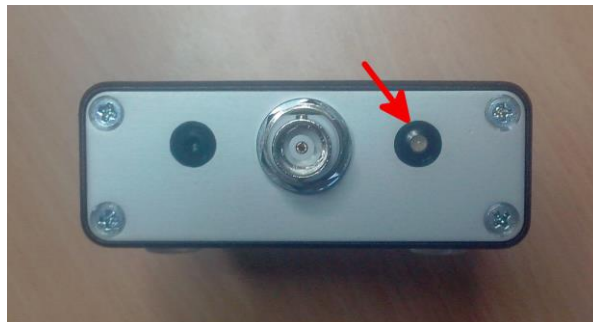
Status LED positioned on the right side of the BNC input. Device is in offline mode. 5
